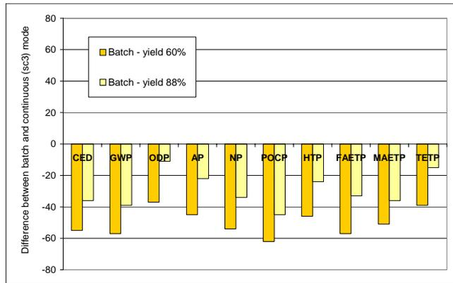
Alterations of each impact category for batch-mode yields of 60 and 88 %, resulting from the transfer to the continuous Cytos® Lab System for the best-case-scenario "cont\_Sc3"
