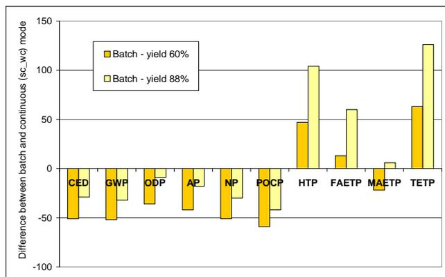
Alterations of each impact category for batch-mode yields of 60 and 88 %, resulting from the transfer to the continuous Cytos® Lab System for the „worst case“-scenario
